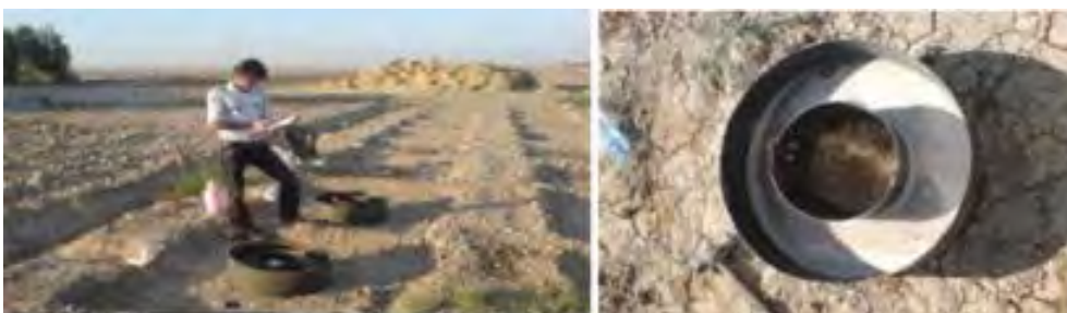
Figure 3.24 Measuring infiltration by double ring method
