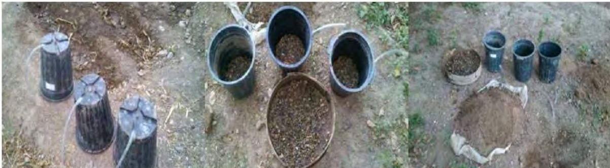
Figure 3.21 Construction, soil preparation, and filling stages in the proposed micro-lysimeter
