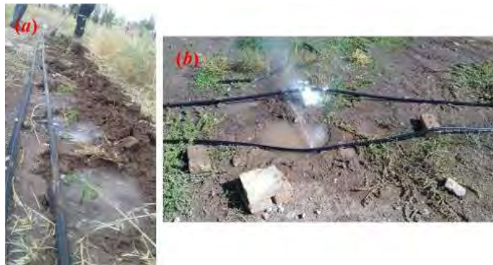
Figure 4.28 (a) No MCOP case with over irrigated areas (b) No MCOP case, tape explosion
