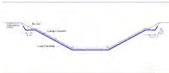
Figure 3.27 GCL installed section underlining of canal
