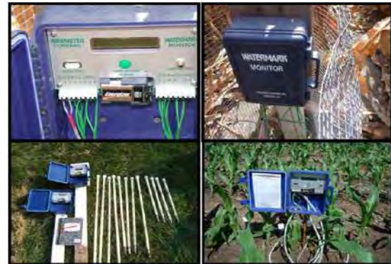
Figure 3.35 Soil moisture sensor devices implemented in the NAWMN
