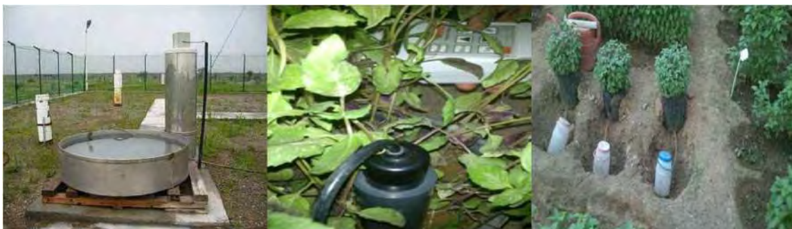
Figure 3.22 View of the proposed micro-lysimeter, Theta probes, and U.S. class-A pan evaporation methods used in the experimental farm
